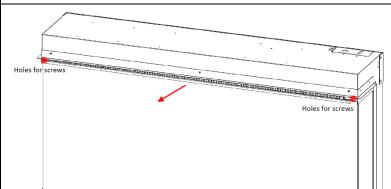
3. Gently lift the glass up and out from the appliance using suction cups and ensuring you have full support of the glass
